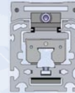
Toothed belt drive with recirculating ball bearing guide
